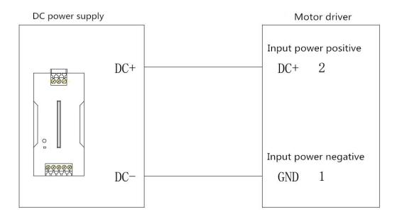
Note 1: The input terminals of the power supply are strictly divided into positive and negative terminals. The voltage range of the input power supply of different models may be different. Please refer to the hardware interface reference wiring of the corresponding model in the section above.
