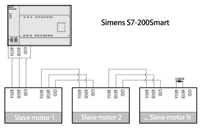
Note 1: Most slave stations are connected. If the communication signal is noisy, it is recommended to add a 120 ohm terminal resistor to the last slave station to ensure the communication quality. Note 2: Communications (4.5 RS485 Parameters)
