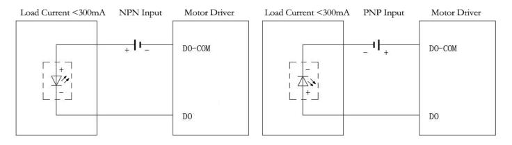
Note 1: The maximum driving capacity of the output terminal is less than 300mA current. If you need to drive a large load, please use intermediate relay to convert.
