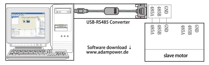
Note 1: Usually there is no direct 485 interface on the computer, so you need to convert USB to 485 to connect the slave motor drive. Note 2: The PC PC debugging software can be downloaded from the official website of our company, which is convenient for users to debug.
