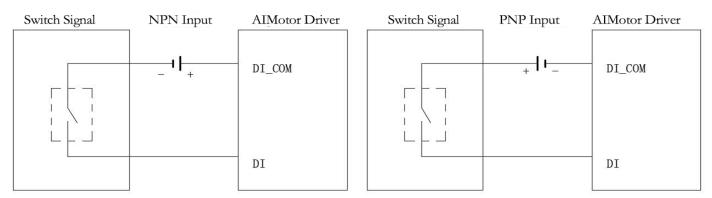
Note 1: The input terminal control voltage DC12-24V is valid;
